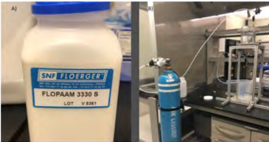
Figure 6—A photo on the left (A) shows the polymer used to make the 1000 ppm polymer solution, while a photo on the right (B) shows the setup for filtering the impurities.
