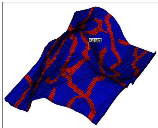
Figure 6.1: The reference model is a channelized system with complex topography. Note that the vertical axis has been exaggerated here for visualization
