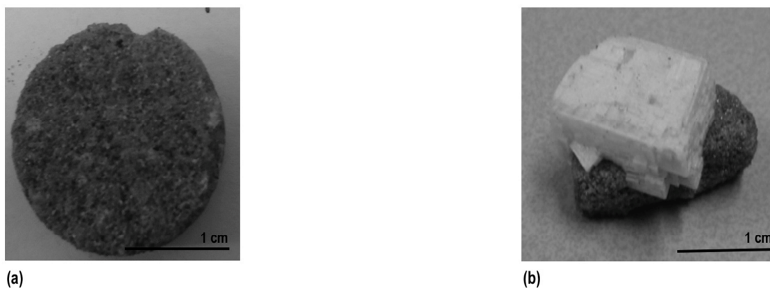
Figure 3.5 The surface of two reservoir samples from the same depth after the experiments. (a) is the reservoir sample after pure CO 2 injection, halite precipitation is not observed on the surface of this sample. (b) The reservoir sample after CO 2 + 5000 ppm H 2 S injection, salt precipitation is observed on the surface of the sample.
