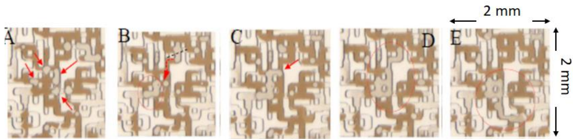
Figure 5-2 micromodel snapshots of (A) formation of third phase bubbles, (B) aggregation of the bubbles to form a third phase batch, (C) combined multiple patches to create a third phase chunk (D and E) third phase chunk displacing the stationary oil blobs during secondary CWI [73]
