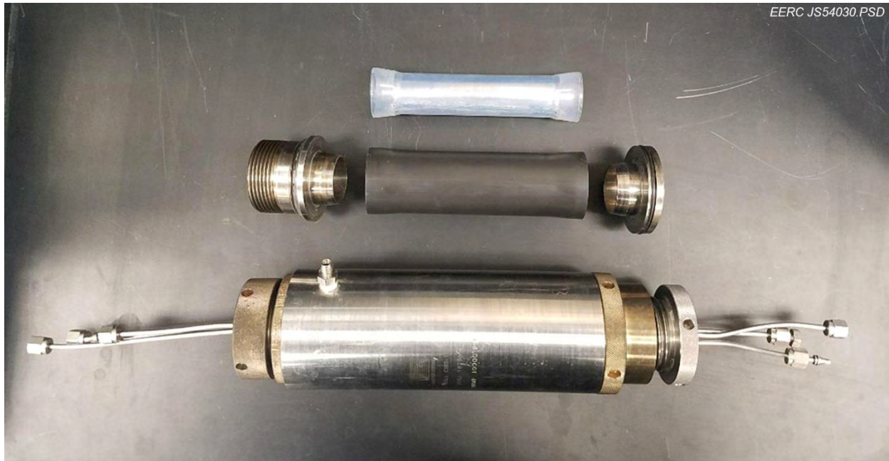
Figure 48. Inner gasket assembly and Hassler-style core holder.
