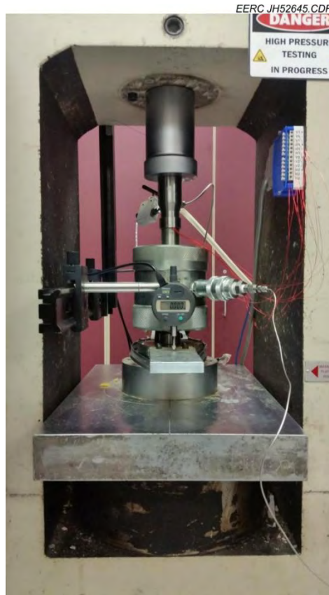
Figure 5. Hoek cell and sample assembly inserted into compression load frame and connected to the system.
