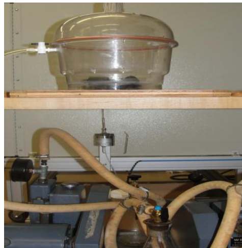
Figure 2.4b Vacuum saturation apparatus
