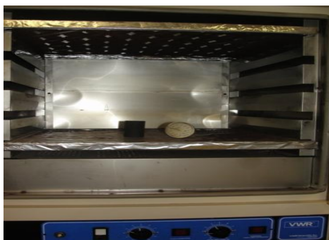
Figure 2.2 Eagle Ford Shale core in an Oven being dried
