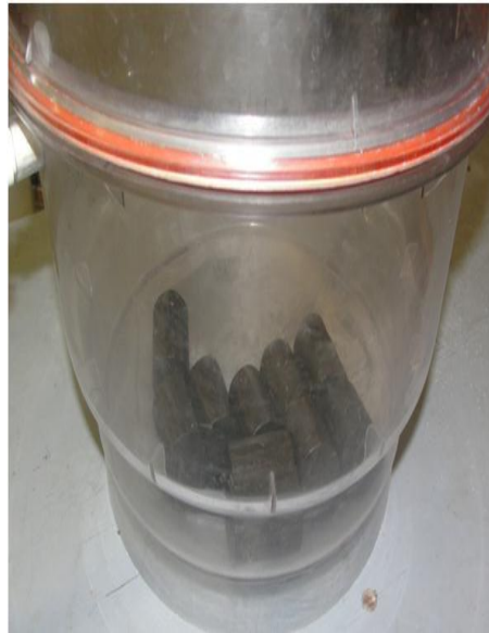
Figure 2.4a Mancos cores in a desiccator being vacuumed
