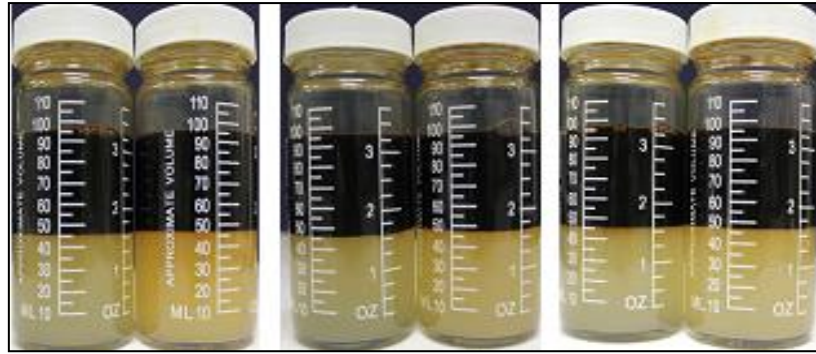
Figure 3.4 Emulsion tendency test results in guar neutral frac fluid with Bakken oil after 5, 15, and 30 min (left: base fluid, right: 0.2 wt% of Stim Aid A)
