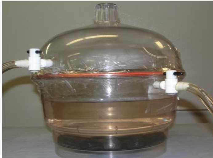
Figure 2.5 Saturation of Mancos core with Soltrol 130 TM Oil
