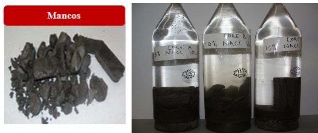
Figure 4.4 Mancos samples in distilled water (the left), and in 5%, 10% and 15% NaCl solutions (the right)
