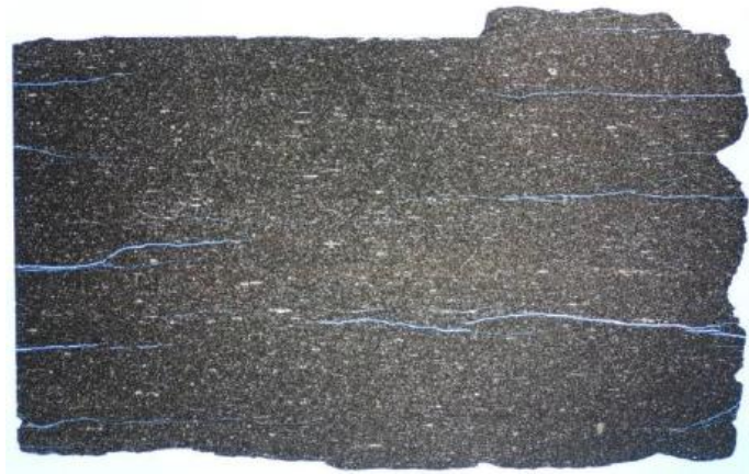
Figure 1.5 Thin section of shale sample exposed in saturated salt drilling fluid (Gomez and He, 2012)
