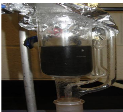
Figure 2.1b Eagle Ford core plug in the soxhlet extractor
