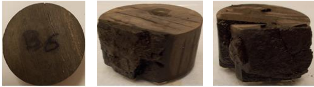
Figure 4.18 Barnett samples after one week of spontaneous imbibition in (a) pH11.9 (0.1 wt% NaOH in Distilled Water) (on the left side), (b) pH11.7 (2 wt% NaOH in Distilled water), and (c) pH12.4 (2 wt% NaOH in 2 wt% KCl) (on the right side)
