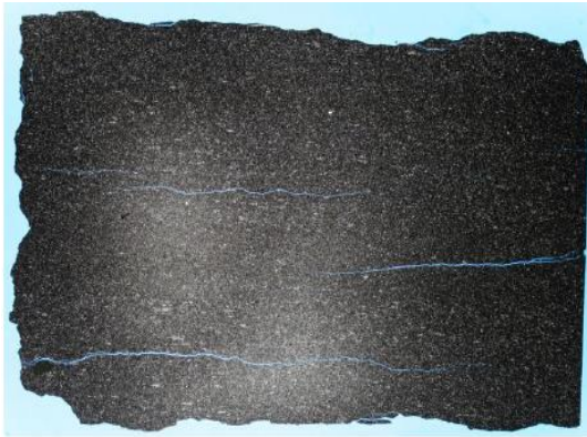
Figure 1.3 Reference shale sample without fluid exposure (Gomez and He, 2012)
