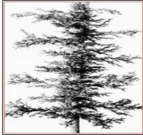
Figure 1.12 Mold of wormholes created by HCl in Limestone from a central conduct after Crowe et al. 1992
