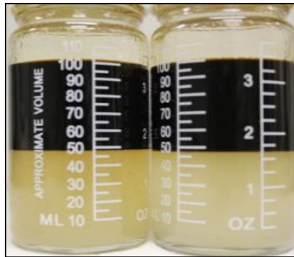
Figure 3.5 Emulsion tendency test Results of 0.2 wt% of Stim Aid A in 15% and 30% brines with Bakken oil after 30 min (left: 15% brine, right: 30% brine)
