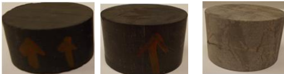
Figure 4.14 Mancos (in the left side), Marcellus (in the middle), and Eagle Ford (in the right side) Shale samples after one week in pH12.4 (2 wt% NaOH in 2 wt% KCl) solution
