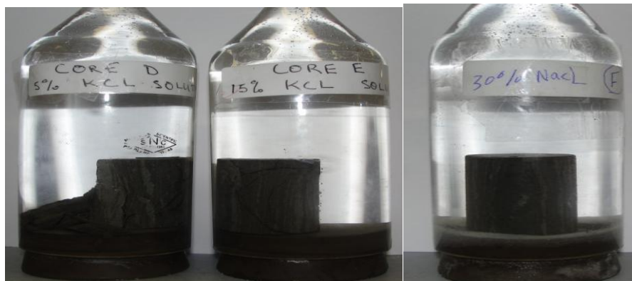
Figure 4.5 – Mancos samples in 5%, 15% and 30% NaCl solutions
