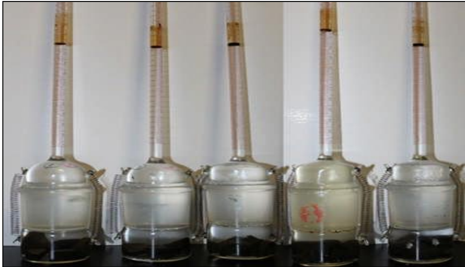
Figure 3.13 Shale cores after 24 hours soaking in the surfactant solutions
