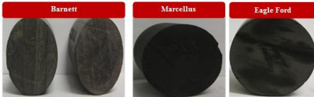
Figure 4.1 Barnett, Marcellus, and Eagle Ford Shale samples after one week of exposure in fresh water
