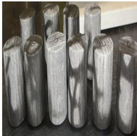
Figure 2.6a Mancos cores after saturation and ready to be weighed
