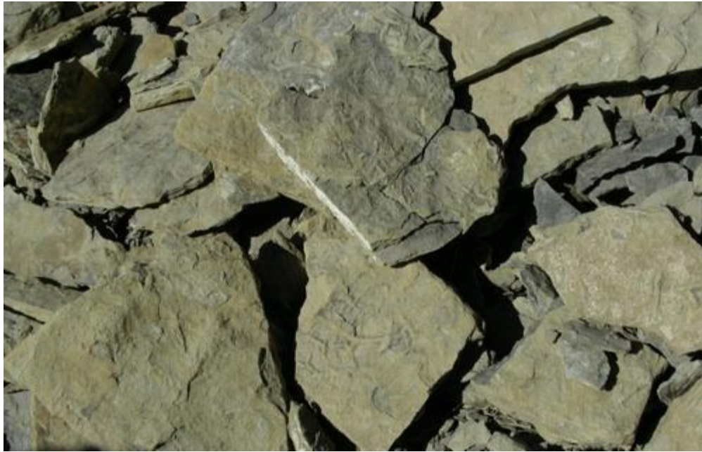
Figure 1.18 Mancos Shale as fissile plates and flakes
