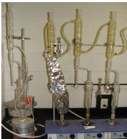
Figure 2.1a Extraction of core sample using the soxhlet extractor
