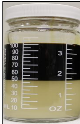
Figure 3.7 Emulsion tendency test result: 0.4 wt% of Stim-aid A in 15% Brine including 0.05 wt% non-emulsifier with Bakken oil after 30 min
