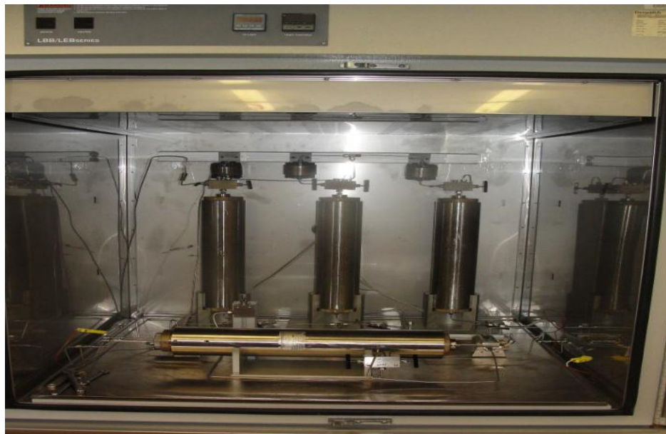
Figure 3.12 Coreflooding system used to saturate Bakken Shale cores prior to water imbibition
